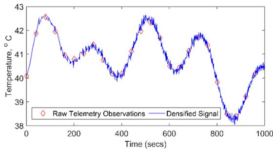
Figure 5. Raw telemetry data and densified signal.
