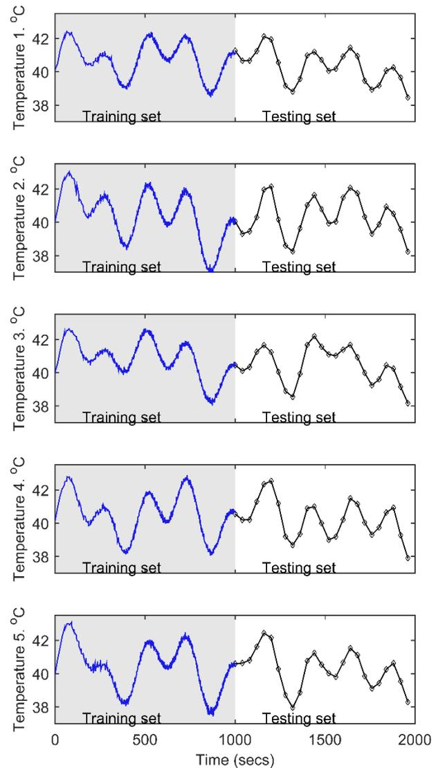
**Figure 3 Training set and testing set of MSET Prognostics**
