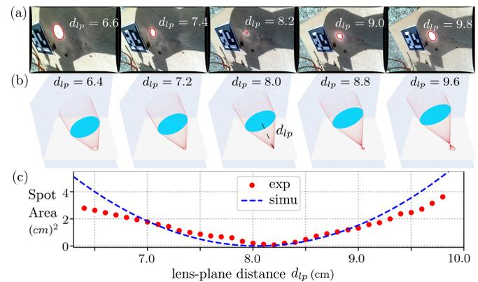
Fig. 10. Image-based focal length calibration experiment. (a) includes snapshots of captured light spot and extracted contour; (b) shows the corresponding lens-plane configuration in the developed simulation; (c) shows the comparison between the light spot area from the real images and the simulation.
