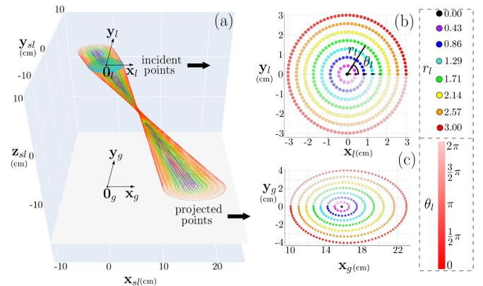
Fig. 5. Illustration of the geometrical characteristics of the projected points. (a) is a simulation of the solar concentration with polar angle  $\varphi_0 = 5/6\pi$  and azimuthal angle  $\theta_0 = 0$ . (b) shows the uniformly sampled incident points on the lens plane. (c) shows the corresponding projected points on the ground plane.
