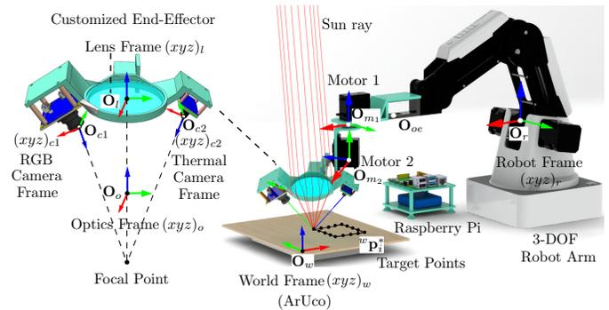
Fig. 3. A schematic of the system with relevant frames. The system is composed of a 3-DOF robot arm with two additional motors (controlled by a *Raspberry Pi*), manipulating a customized end-effector. The end-effector carries a spherical Fresnel lens, an RGB camera, and a thermal camera. An ArUco marker defines the World Frame.
