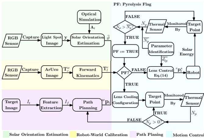
Fig. 2. Workflow of the proposed robotic painter.
