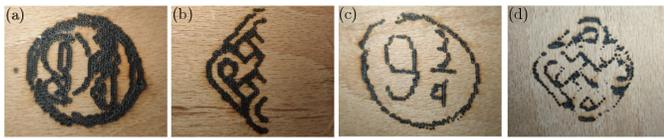
Fig. 15. Examples of failed solar paintings, which are caused by (a) inappropriate feature selection in the path planning stage, (b) the lens being shadowed as the solar orientation changed, (c) inaccurate solar orientation estimation and (d) a cloudy situation when  $N_p$  is set too small.
