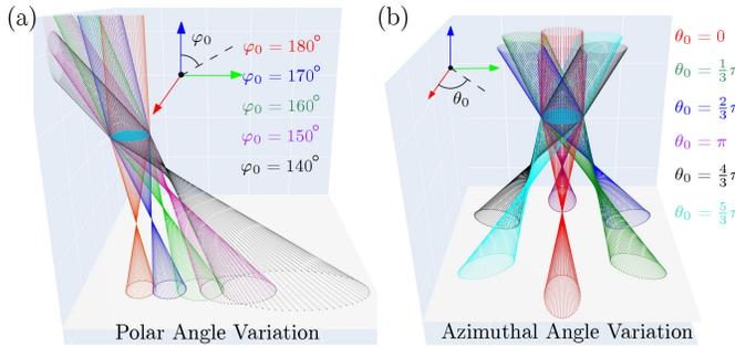
Fig. 6. The effect of the solar orientation variation on the light spot when the lens plane is parallel to the ground plane. (a) shows the effect of the variation of the solar polar angle  $\varphi_0$ . (b) shows the effect of the effect of the variation of the solar azimuthal angle  $\theta_0$ .
