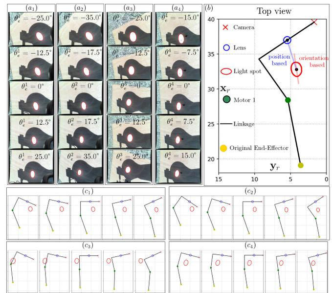
Fig. 11. Experiments evaluating the performance of the solar orientation estimation utilizing different geometric features. (a<sub>1</sub>)–(a<sub>4</sub>) include images captured from four experiments with varying lens yaw angles, and (c<sub>1</sub>)–(c<sub>4</sub>) show the corresponding robot configuration from the top view. (b) annotates the components in the robot configuration visualization.
