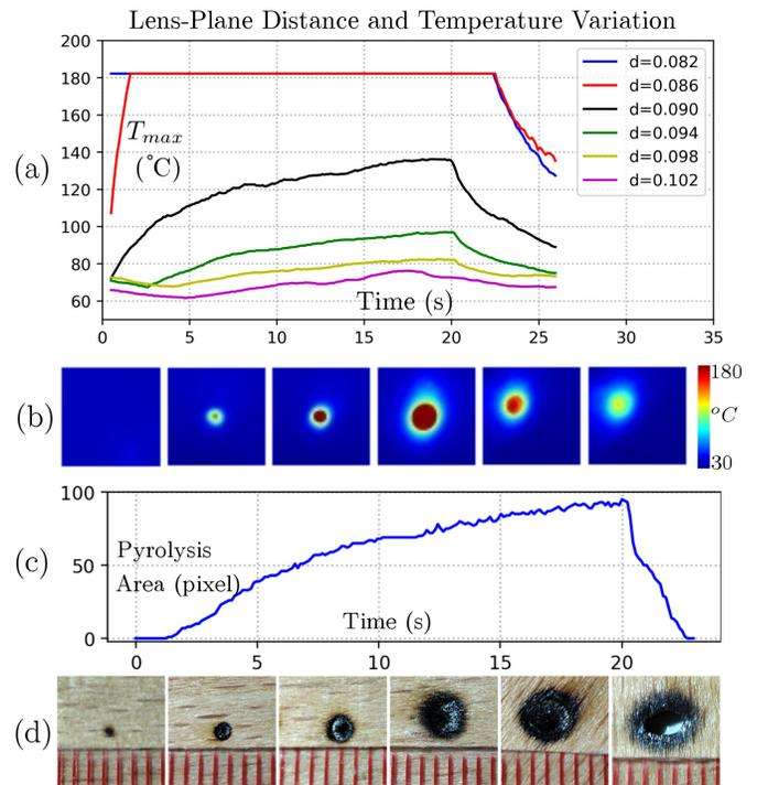
Fig. 8. Experiments designed to determine the parameters for the motion control algorithm. (a) Solar concentration experiments with fixed duration and varying lens-plane distance. (b) Representative thermal images captured before, during and after the wood pyrolysis process; (c) Variation of the pyrolysis region with respect to time when the lens-plane distance is set to 0.086 m; (d) The size of a carbonized point can be controlled by the selection of  $\bar{N}_p$ .
