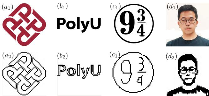
Fig. 9. Feature extraction and scaling from target figures for path planning. The obtained target points were used for conducting real solar painting experiments as reported in Sec. V-C.
