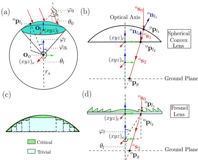
Fig. 4. Ray tracing and structure diagrams of the plano-convex lens and the Fresnel lens.
